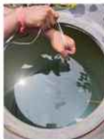
Hour meter were submerged in water at a depth of 1 meter
